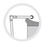
Due to the pool's sloped edge (coping), the pad on the support bar does not have contact with the surface. Therefore, the EdgeMate Pool Chair will NOT hold a stationary position.
